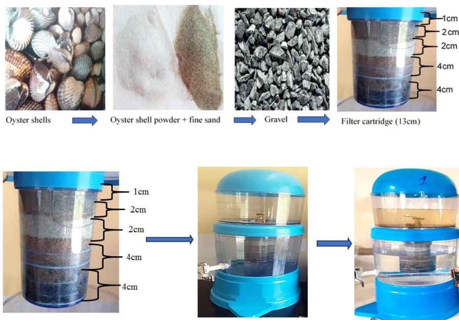
Figure 1. Experimental water purification device designed (intermittent biosand filter amended with oyster shell powder).
